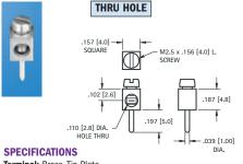
Terminal: Brass, Tin Plate Screw: Steel. Zinc Plate Mounting Hole: .047 (1.2) **Current Rating: 15 AMP**
