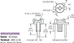
Brass, Matte Tin Plate Screw: Steel. Nickel Plate
