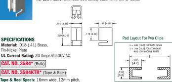
HORIZONTAL ENTRY For Mini: Littelfuse: MIN series/ Bussmann ATM series or equivalent
