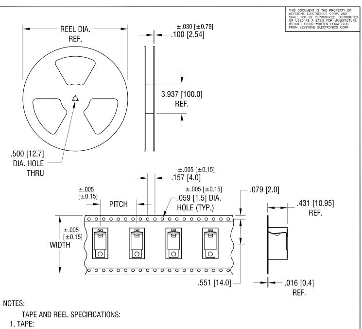
MAT'L - ALL CONDUCTIVE POLYSTYRENE CARRIER ANSI/EIA-481 STANDARD 1.260 [32.0] WIDE; .787 [20.0] PITCH
